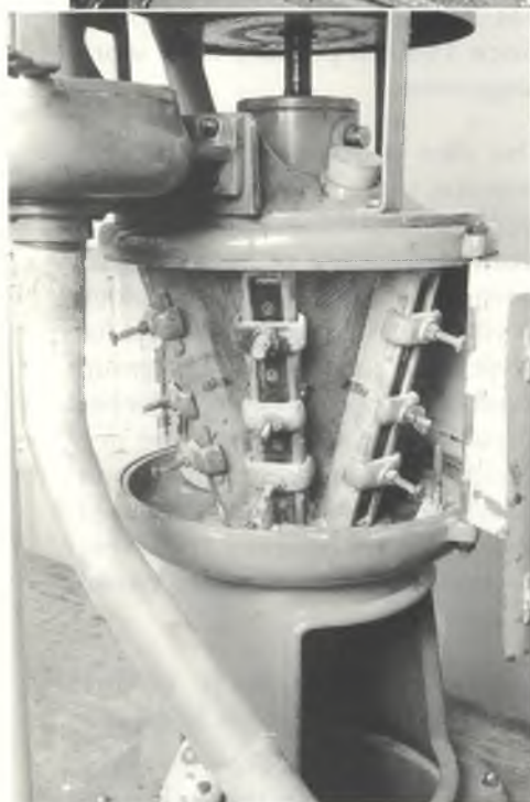
The blancher. After several runs, the mill cone gradually wears down the outer caryopsis layer of the cargo rice grain to obtain white rice.
