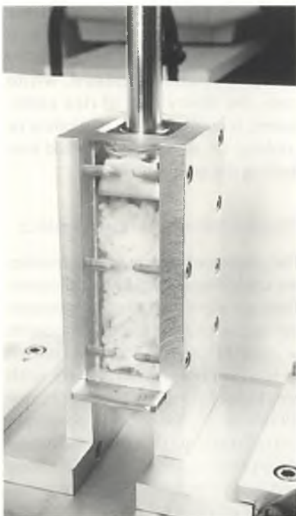
Measuring firmness in cooked rice with an Instron texturometer.
