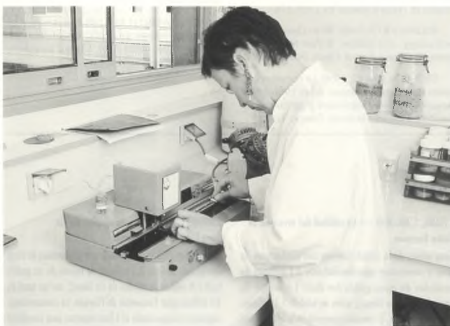
Semiautomatic measurements of rice grain lengths/widths using a Russian HP3-8 apparatus.
