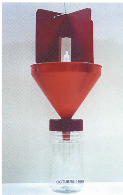
Photo 2. Prototype B of the trap, precursor of the Brocap® trap.
