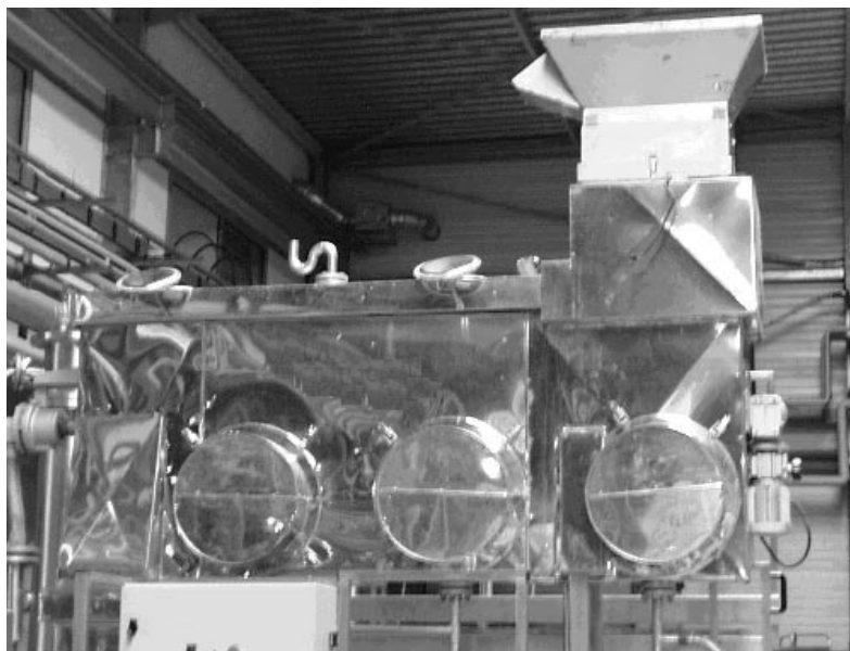
Figure 1. Steam-heating chamber of the flash vacuum-expansion process (with the permission of FABBRI SA, 84320 Entraigues, France).
