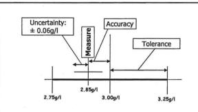
Uncertainty should be lower than 1/4 of tolerance Tolerance should be higher than 3 x accuracy
