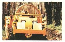
Subsoiling before trees are felled in an old oil palm plantation being prepared for replanting.
