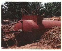
Transpaille, a fermentor that continuously processes hay to produce energy and compost.
