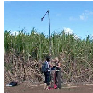
Fig.3: In-situ measurements of surface temperature using a hand-held infrared thermometer HEITRONICS KT19 ® mounted on a mast.
