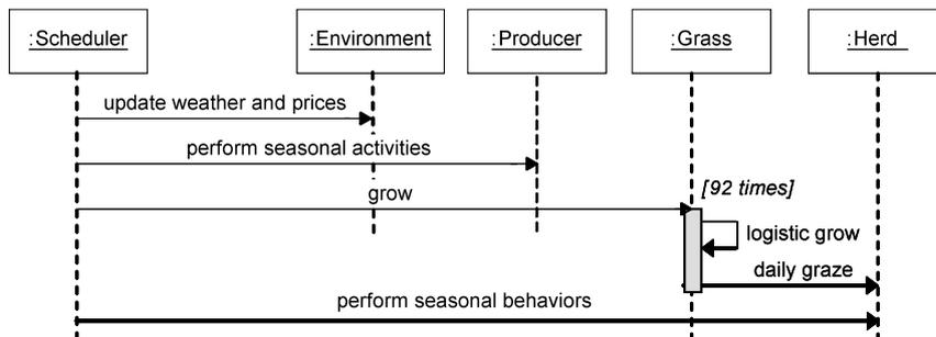
Fig. 3. UML Sequence diagram representing task scheduling of a seasonal step
