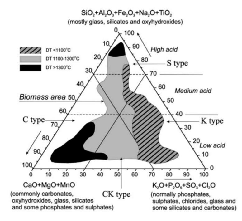
Areas of low, medium and high initial deformation (DT) ash fusion temperatures for 55 varieties of biomass. Vassilev et al. (2014)
