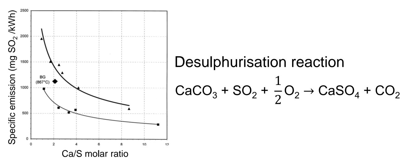
Specific SO<sub>2</sub> emissions as a function of Ca/S molar ratio of blended fuel pellets (lignite, wood, lime) for 2 grate temperature (upper curve: 1000°C; lower curve: 800°C). Heschel et al. (1999)
