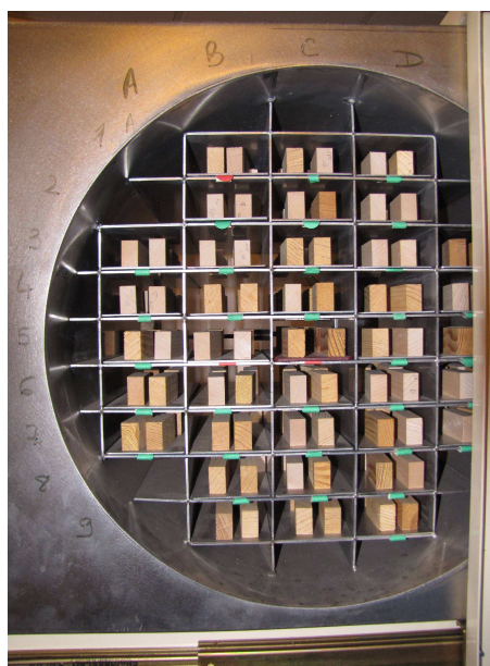
Figure 3. Outlet of the compartments of the wind tunnel with once calibration is done.
