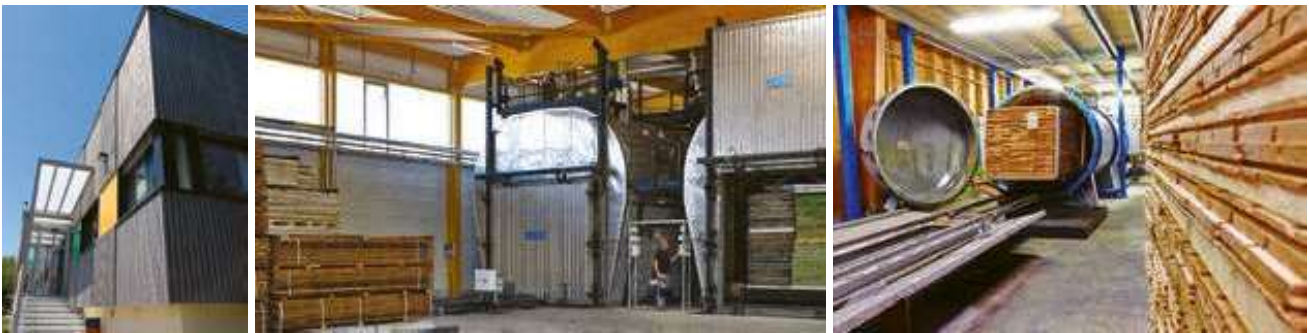
Figure 23: The use of modified wood in France: siding of thermally modified poplar wood by Bois Durable de Bourgogne® company (left), thermal-modification kiln, Jartek®, 20 m 3 , Bois Durable de Bourgogne® (middle), and WoodenHa® process, fire-retardant impregnation in an autoclave (right).
