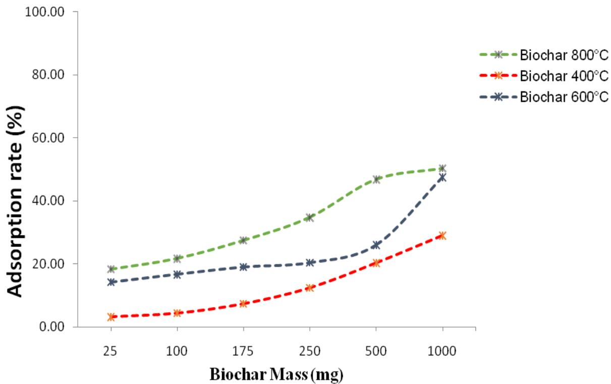
Figure 3. Ochratoxin A adsorption by filtration method using three different biochars (400, 600 and 800°C) at pH 6.54.
