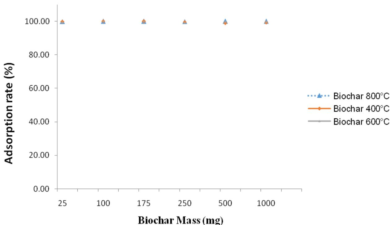
**Figure 8.** Aflatoxins adsorption test results by stirring method using three different biochars (400, 600 and 800°C).
