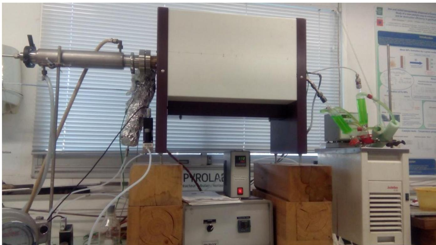
**Figure 1.** Biochar production equipment.
