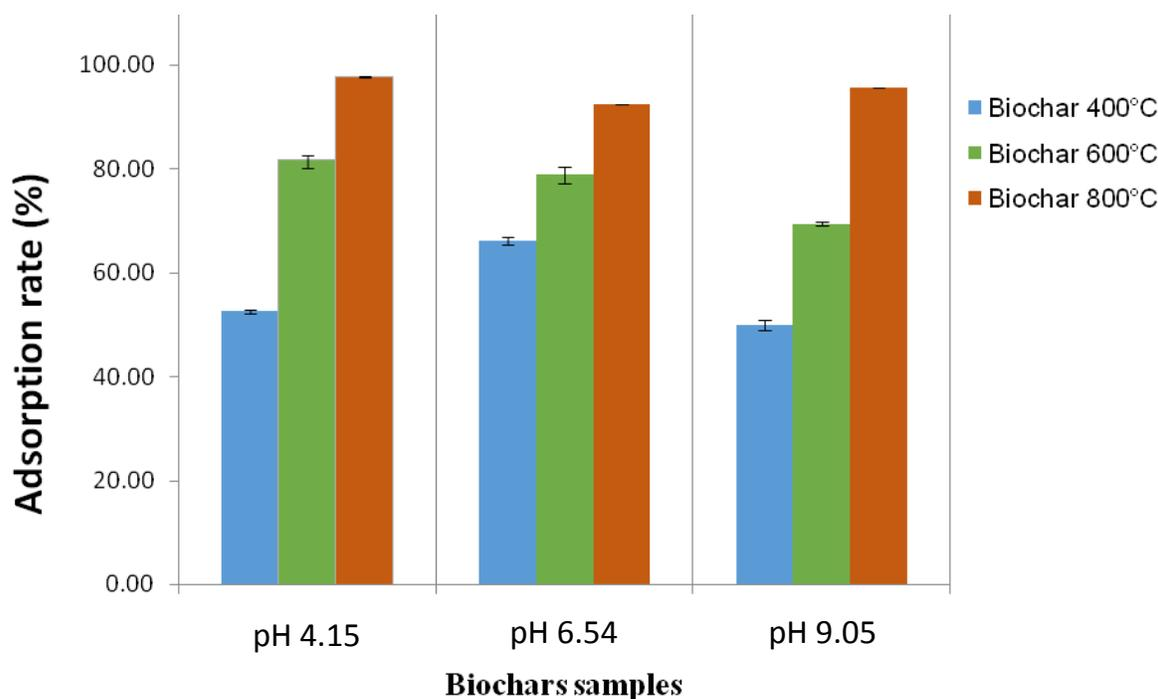
**Figure 5.** Ochratoxin A adsorption results by stirring method using three different biochars (400, 600 and 800°C) under different pH conditions.
