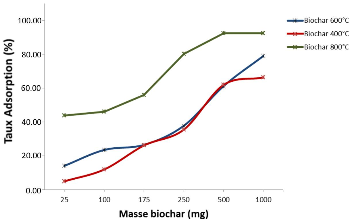
Figure 4. Ochratoxin A adsorption results by stirring method using three different biochars (400, 600 and 800°C).
