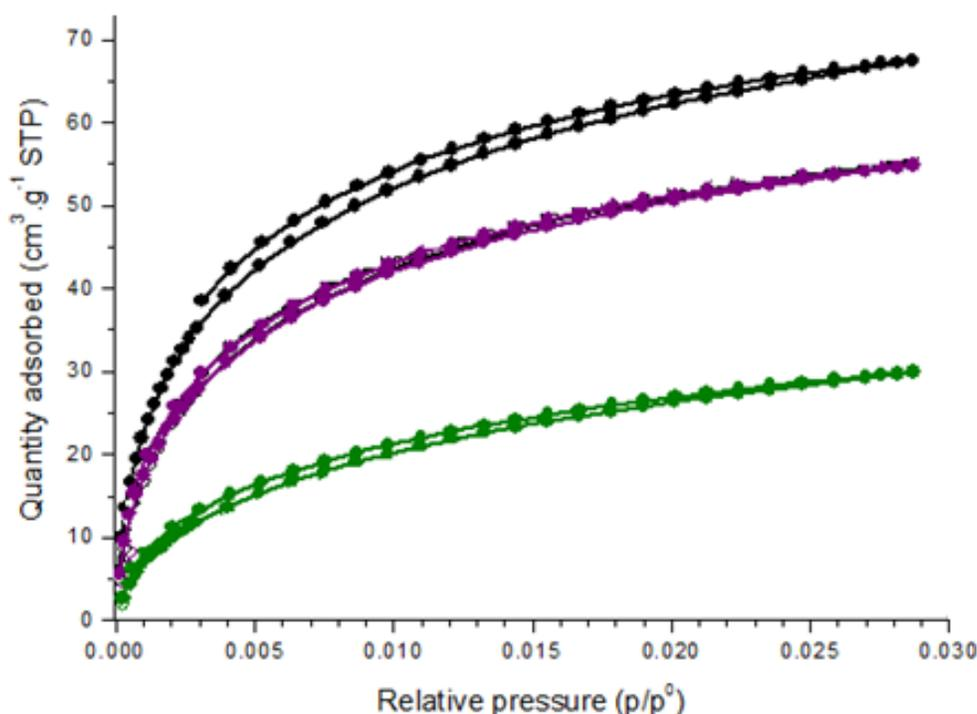
**Figure 2.** Influence of pyrolysis temperature on CO<sub>2</sub> adsorption by different biochars.
