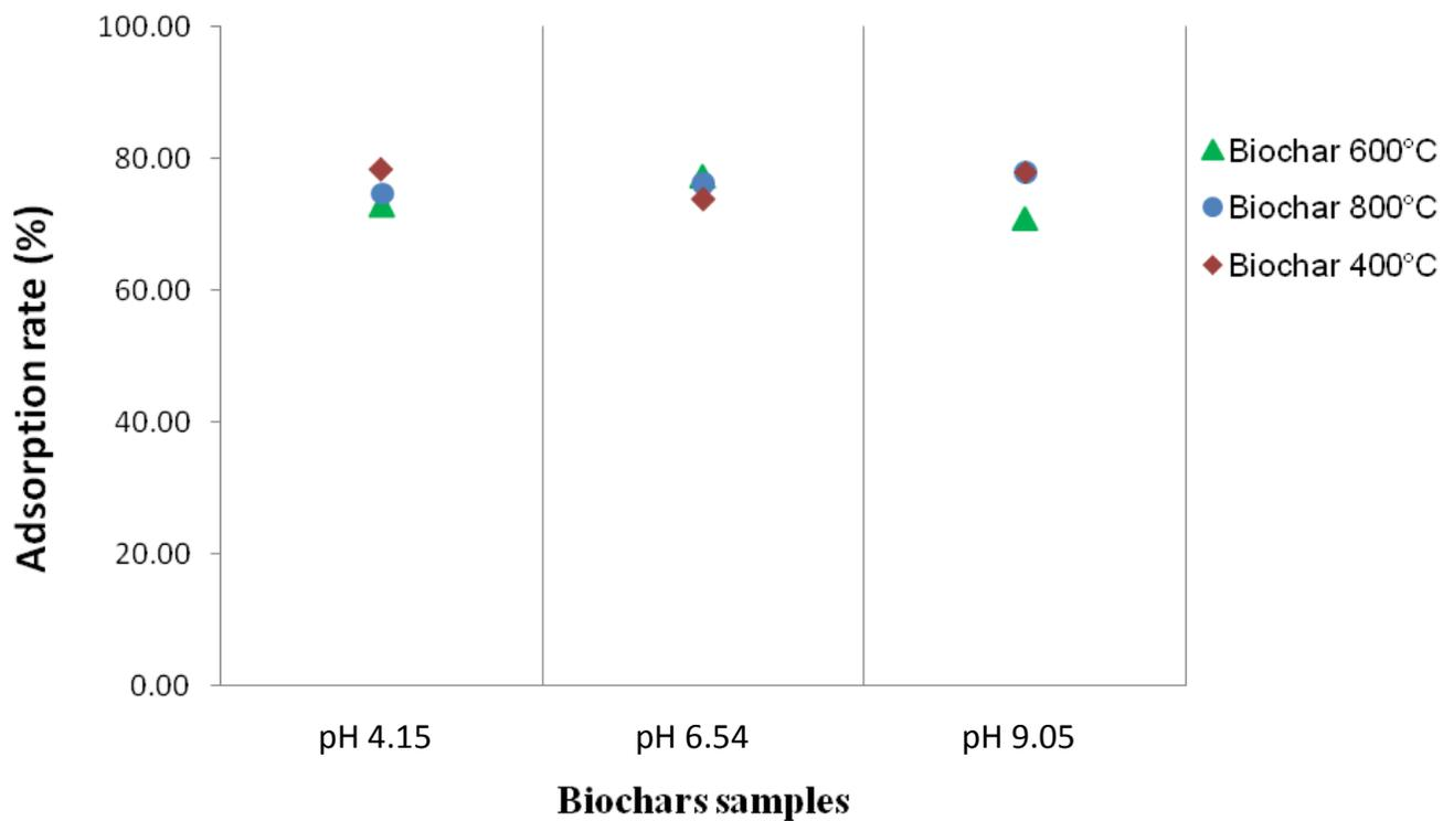
Figure 7. Aflatoxins adsorption results by filtration method using three different biochars (400, 600 and 800°C) under different pH conditions.
