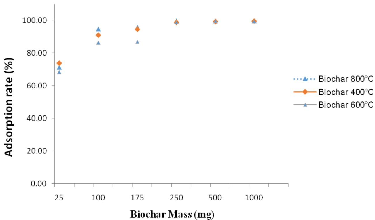
Figure 6. Aflatoxins adsorption test results by filtration method using three different biochars (400, 600 and 800°C).
