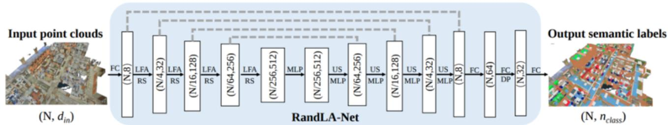
Figure 7. The detailed architecture of our RandLA-Net.  $(N, D)$  represents the number of points and feature dimension respectively. FC: Fully Connected layer, LFA: Local Feature Aggregation, RS: Random Sampling, MLP: shared Multi-Layer Perceptron, US: Up-sampling, DP: Dropout.
