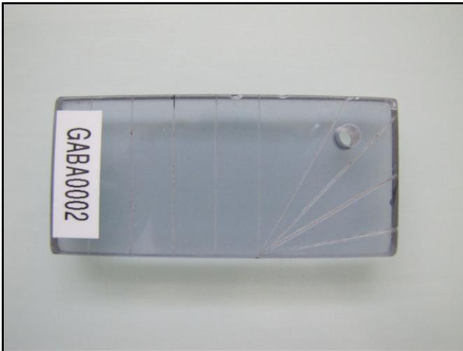
Fig. 1. Test gauge for wood sample selection ( $\pm 1$  mm,  $\pm 1^\circ$ ).
