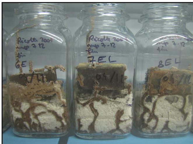
Fig. 7. Culture flasks (test device) with termites.
