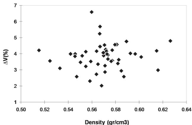
FIGURE 2. Relationship between change in volume  $\Delta V\%$  (between air dried and 60 °C/ 48 h) and density (measured at 60 °C/ 48 h) for 60 samples before submitting to treatment.
