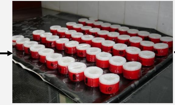
DGT deployment on different combinations after 0, 7, 14 and 28 days mineralization at 28 °C
