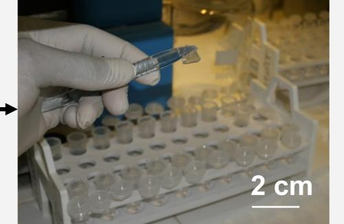
Extraction of resin binding gel from DGT
