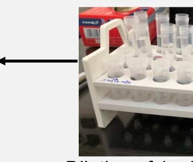
Dilution of 1 ml of elution solution in 7 ml of demineralized water
