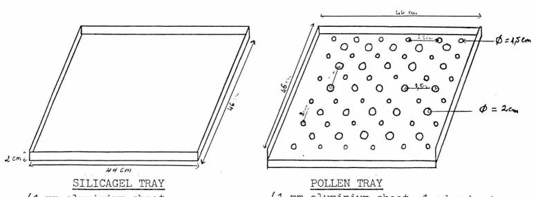
(1 mm aluminium sheet, 1 edge bent downwards to make it easier to remove pollen). (1 mm aluminium sheet, 4 raised edges)
