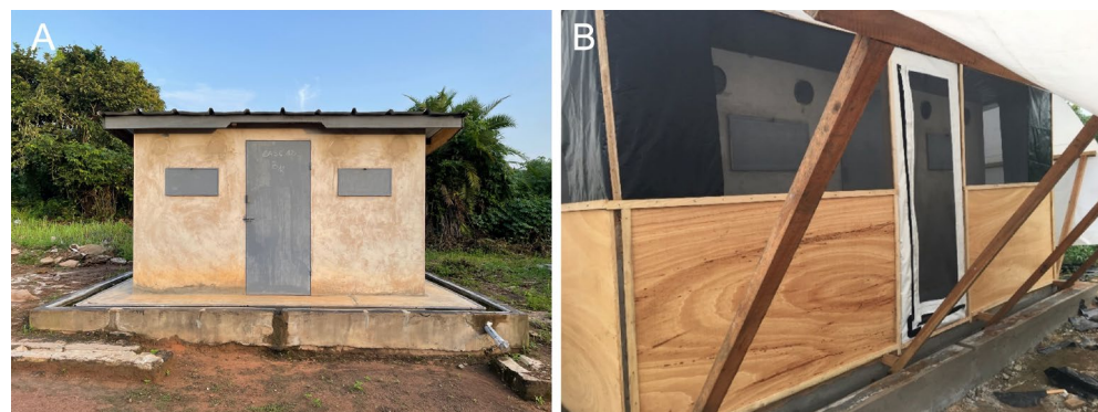
Figure 1. (A) West African experimental hut style at the M'Be rice field, central Côte d'Ivoire, (B) West African experimental hut fitted with eave tubes and surrounded with an enclosure.
