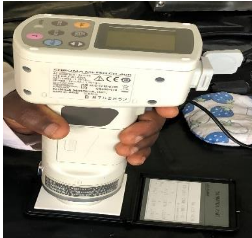
Figure 2: The measuring head of the Chroma Meter placed on a white calibration tile.
