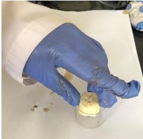
Figure 6: The pulp sample being placed into a precision cell.
