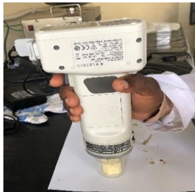
Figure 7: The measuring head focused on the precision cell.
