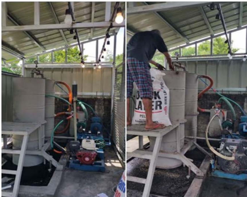
The figures above are for the ARB Biomass Gasifier developed at PhilRice. It can drive stationary agricultural machines such as a 4-in. pump, a 30-cm biomass chipper, and a 20-cm rubber creeping mill. It can also power a 3-kWe AC generator for lighting and a 60-Amp DC alternator for charging batteries. [19]
