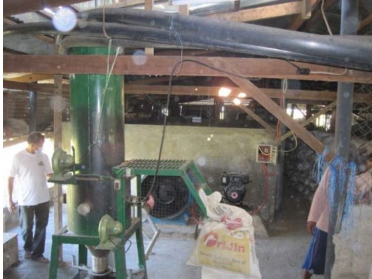
The CFRHG Model-40D Used for Drying Paddy Seeds in Nueva Ecija, Philippines [18].
