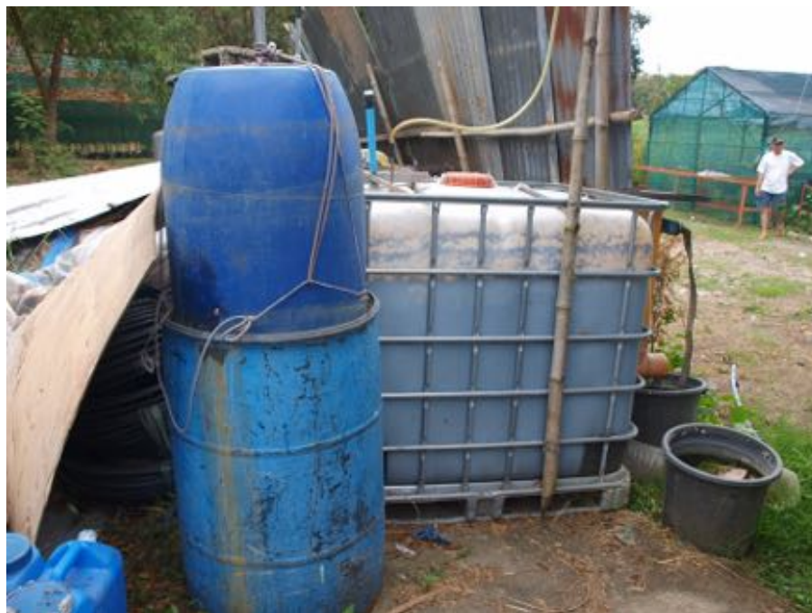
Floating Drum Digester at the Pampanga Agricultural College [32]
