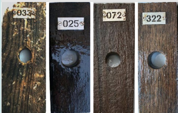
033: Scots pine ( Pinus sylvestris ) after 1 year 025: Acaria ( Minquartia guianensis ) after 22 years 072: Azobe/Ekki ( Lophira alata ) after 8 years 322: Angelique ( Dicorynia guianensis ) after 6 years
