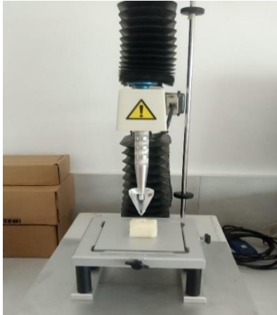
Figure 5 : Example of penetration test set-up
