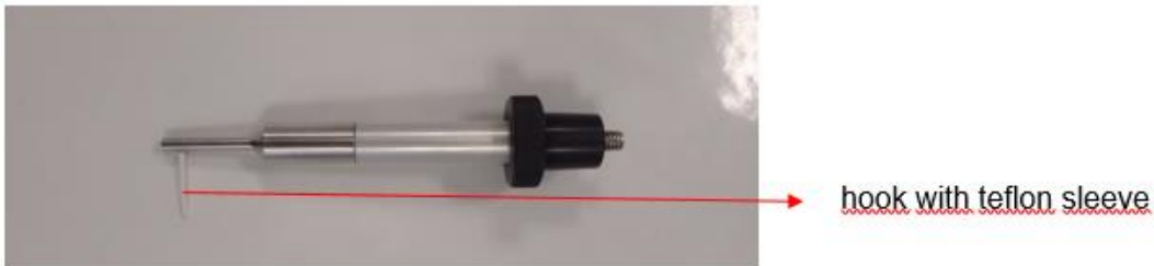
Figure 3 : Kieffer probe with teflon sleeve
