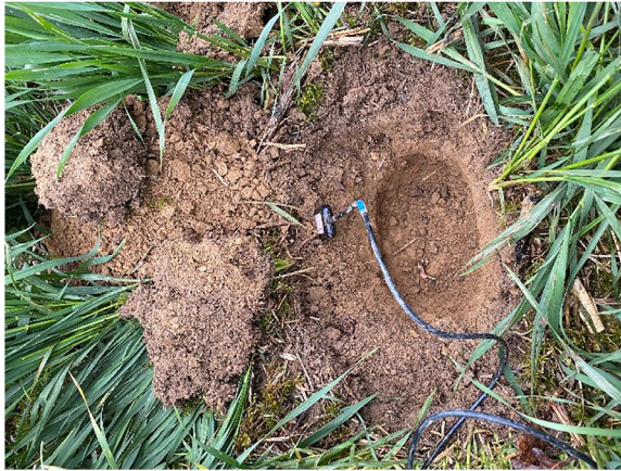
Photo 1. WET sensor on a CA plot, after VESS measurement. WET sensors measurements were done on the non-disturbed part of the VESS measurement square. Note the visible darker soil colour in the superficial horizon. © Clara Lefèvre, April 2023.
