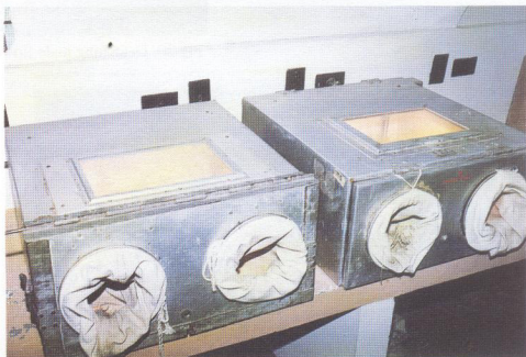
Fig.18. Sterilization of Pollen Manipulation Box (PMB) using two infra-red lamps (1000 watt per bulb)
