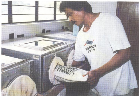
Fig.19. Transferring spikelets with male flowers into the PMB
