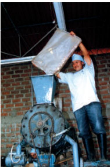
Loading a preheating module prior to a continuous oil pressing operation. Lima, Peru.
