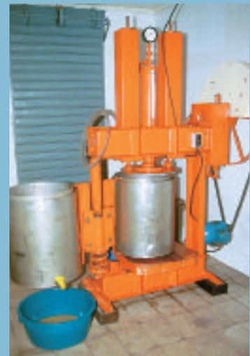
Oil production. Handmade hydraulic press (batch pressing). Laranjal do Jari, Brazil.
