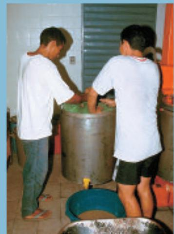
Oil production. Loading a hydraulic press (batch pressing). Laranjal do Jari, Brazil. Photo D. Pioch.
