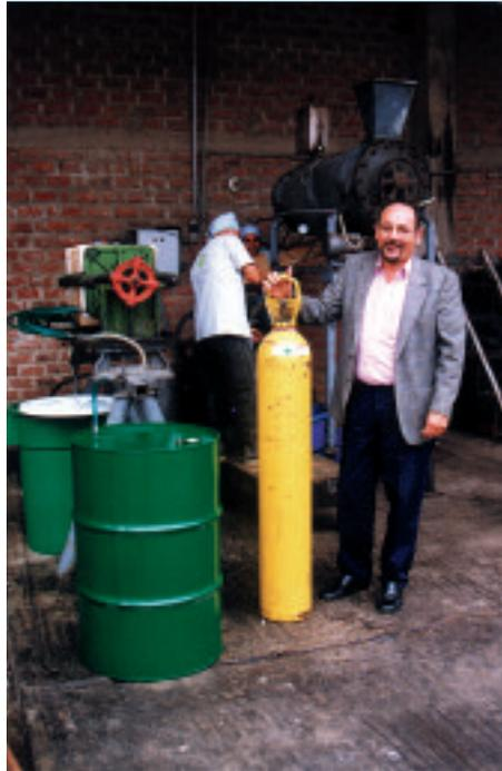
Storing oil in 200 l barrels, in an inert atmosphere, prior to export. Lima, Peru.
