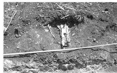
Poor compacted soil in northern Grande-Terre, Guadeloupe. © C. Poser
