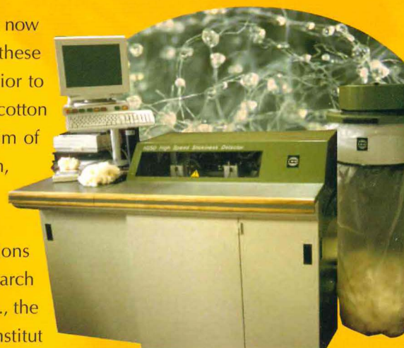
H2SD (high-speed stickiness detector). © R. Frydrych Background photo: Microscopic view of aphid honeydew on cotton fibre. © CIRAD
