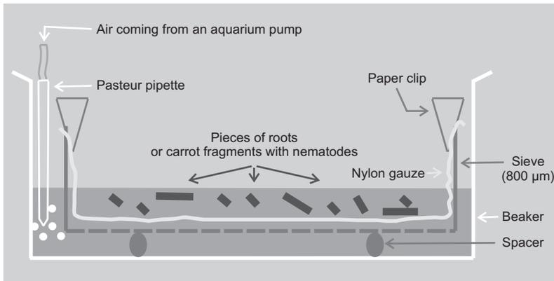
**Figure 1.** Device allowing the collection of nematodes from carrot fragments after their inoculation in petri dishes.
