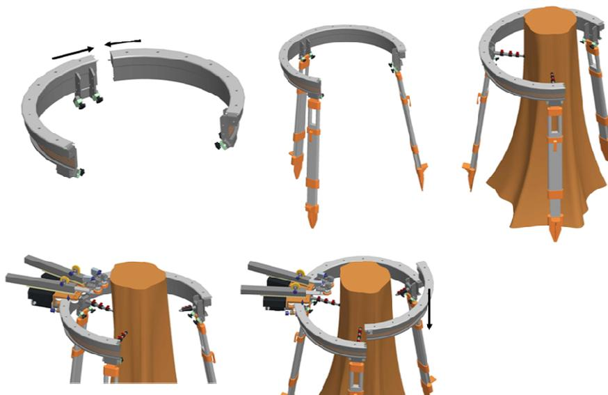
Fig. 1 Schematic view of the device assembly.
