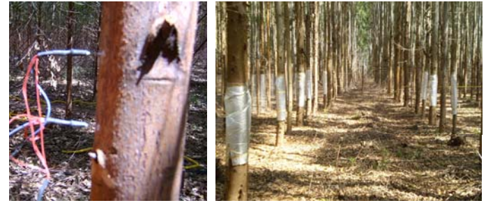
Figure 4. View of the sapflow sensors placed in the trunk of Eucalyptus trees.
