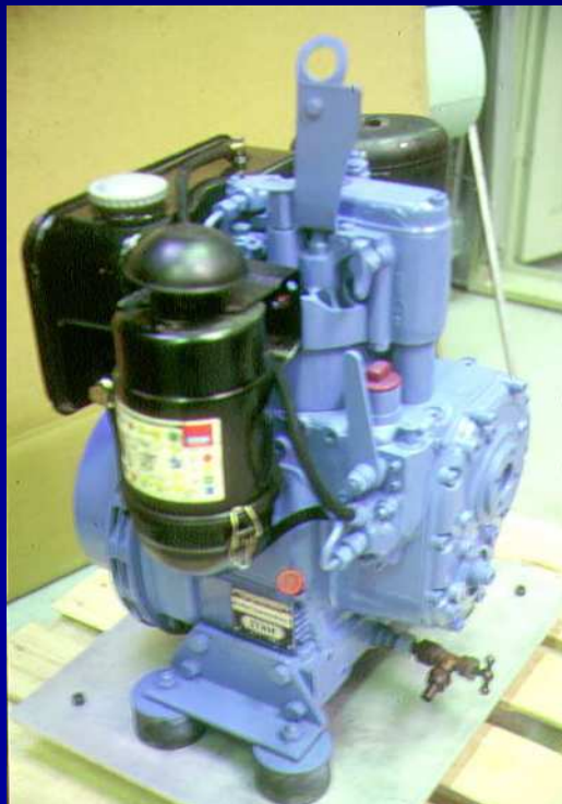
HATZ ENGINE TO BE COUPLED TO 7 KVA GENERATOR (FUELED WITH COCONUT OIL, FIDJI )
