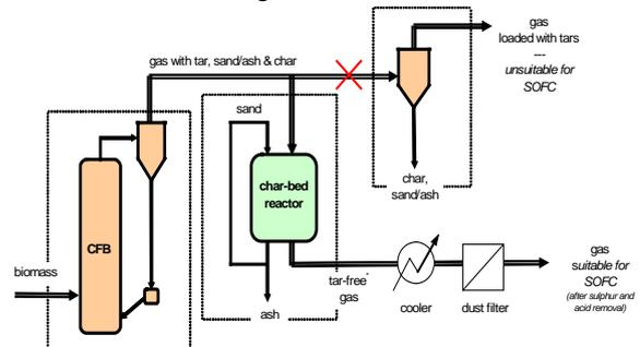
**Figure 6:** Schematic positioning of the TREC reactor downstream the gasifier (ECN).
