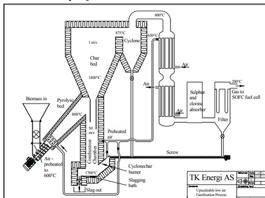
**Figure 5:** TKE upscalable staged gasifier
