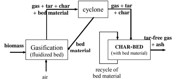
**Figure 4:** ECN concept of char bed for tar removal
