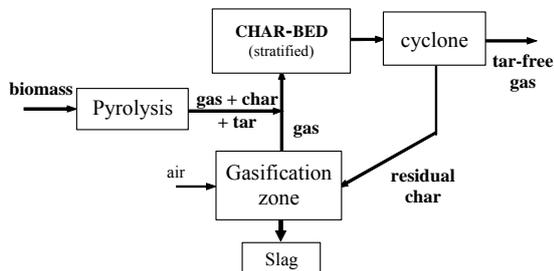
**Figure 3:** TKE concept of char bed for tar removal
