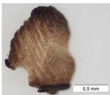
Figure 16: Wood particle after pyrolysis (T=1073 K; solid residence time = 0.45 s)
