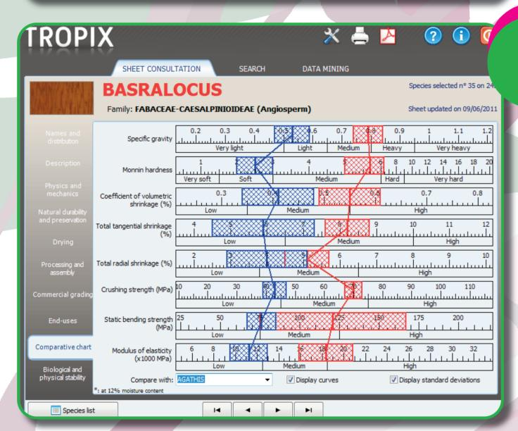
graphical comparison of the main physical and mechanical properties and a schematic summary of the main parameters of physical and biological stability.
