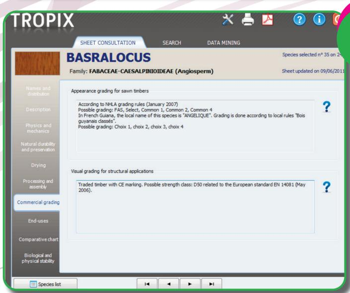
commercial grades: appearance grading of sawn timbers according to the existing rules and visual grading for structural applications
