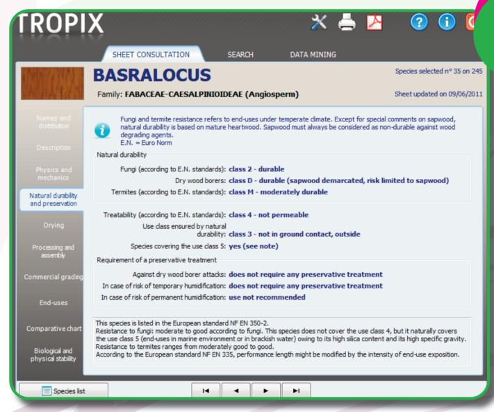
Resistance of wood to biological agents of deterioration (fungi, termites, dry wood borers), impregnability, use classifications, any conditions for preservative treatment according to the conditions of use.
