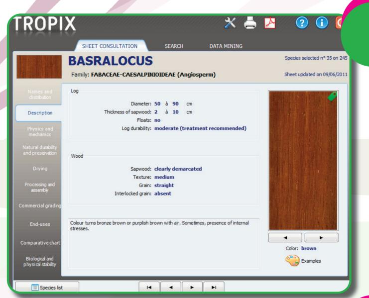
Characteristics of logs: appearance, color and macroscopic structure of wood, illustrated with pictures of wood and examples of use.
