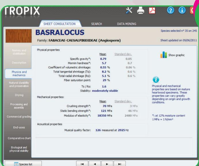
Main physical and mechanical properties such as specific gravity, hardness, stability, shrinkages, crushing and static bending strengths, modulus of elasticity and acoustical quality.
