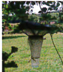
Figure 1. An Onderstepoort type down draught black light trap, fitted with UV bulb.
