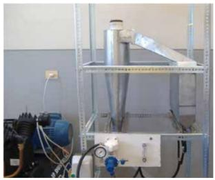
**Figure 24:** Spouted bed reactor for dry saponin removal (Courtesy of UPB)
