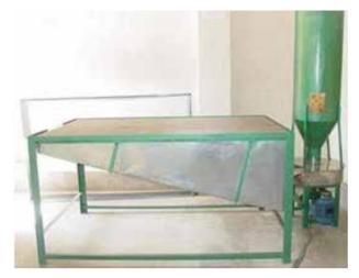
Figure 31: Warm air generator (Courtesy of: CPTS)
