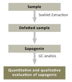
Figure 2: Schematic diagram for the extraction of saponins
