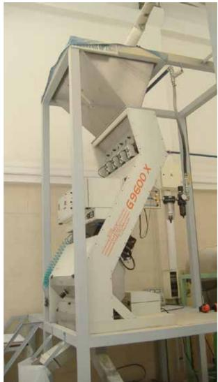
Figure 34: Optical-pneumatic sorter (Courtesy of: CITY and UPB)
