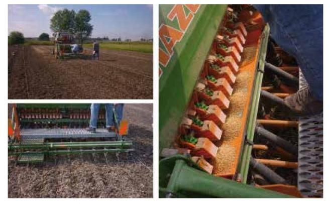
Figure 9. Mechanization of quinoa sowing
