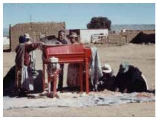
Figure 10: Tubular thresher (Source: Fundación PROINPA 2008)
