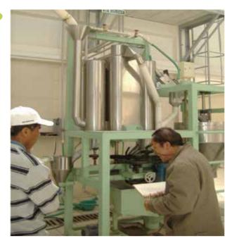
Figure 29: Wet cleaning system (Courtesy of: CITY and UPB)
