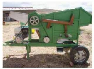
Figure 9: The modified Vencedora thresher (Source: Fundación PROINPA 2008)
