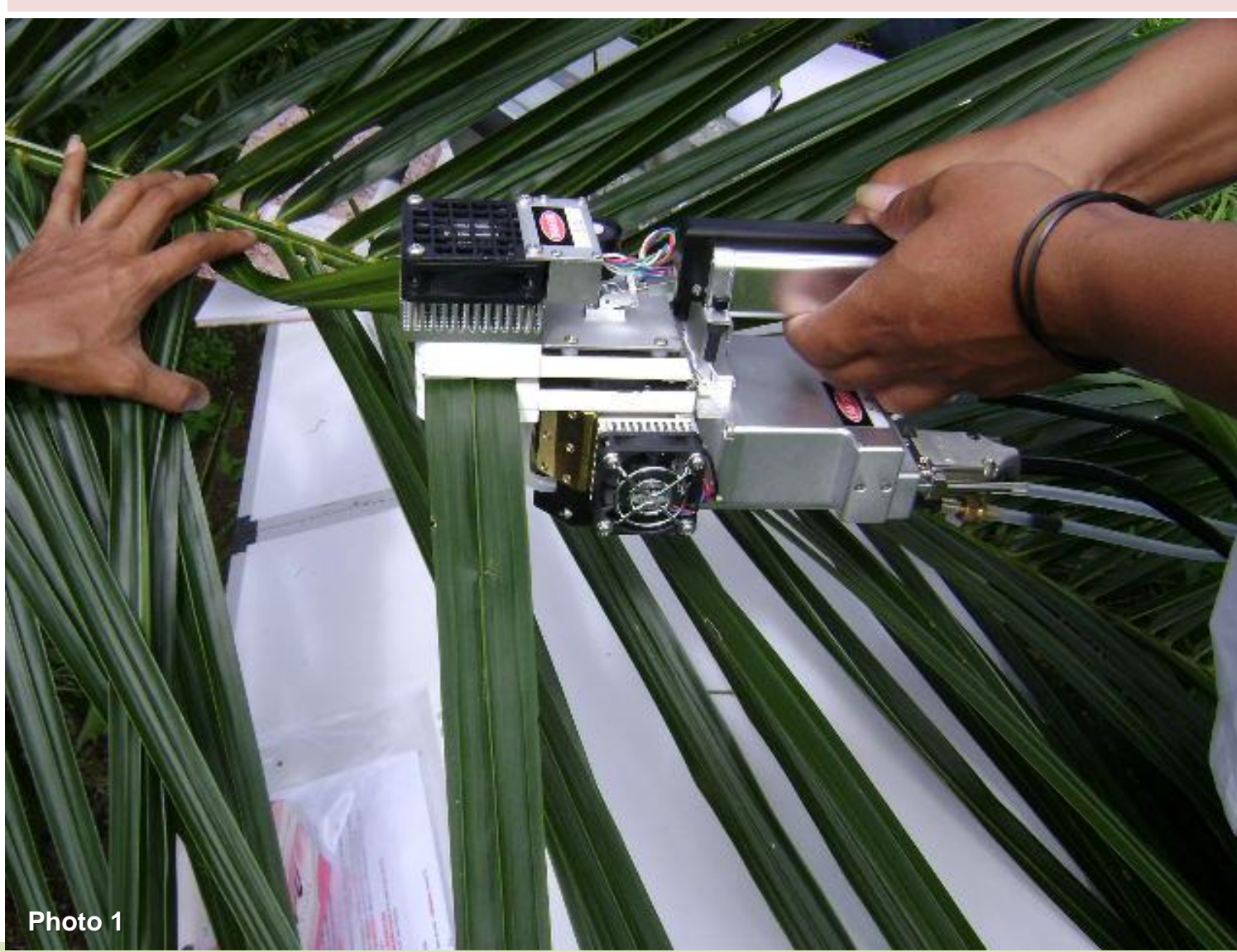
Photo 1 Leaf gas exchanges study with the Licor 6400 on oil palm leaf at Bah Birung Ulu Estate, North Sumatra.
