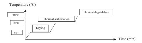
Figure 1. Temperature evolution to achieve thermal treatment.
