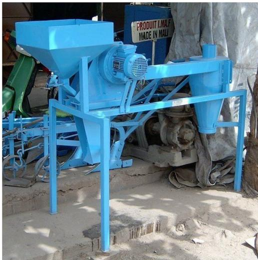
Figure 19: Canal de vannage (© C. Marouzé, Cirad)
