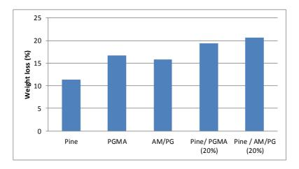
Figure 1. Weight losses recorded after 2 hours at 220°C by thermo gravimetric analysis.
