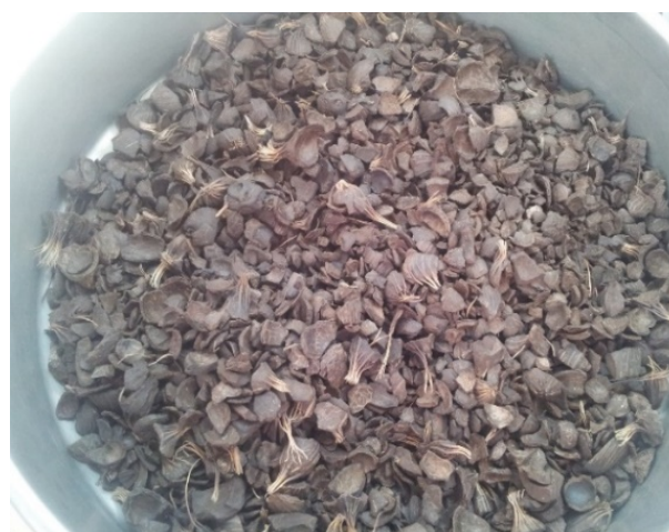
Fig. 1 Sample of OPS aggregate.
