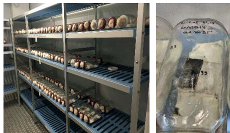
Figure 2: Samples exposed to Coriolus versicolor following the EN 113 standard procedure
