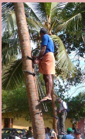
Coconut palm climbing mechanical device in India. (A. Prades, CIRAD)
