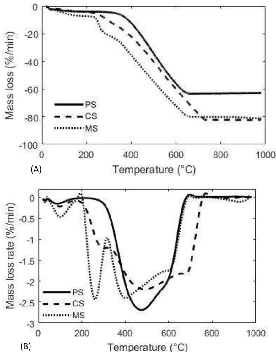
**Figure 2.** (a) Mass loss from thermogravimetric analysis of coal briquettes (b) Mass loss rate from thermogravimetric analysis of coal briquettes.
