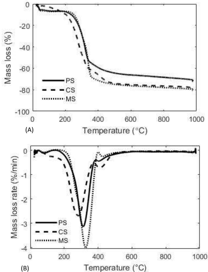
**Figure 1.** (a) Mass loss from thermal decomposition (TGA) of biomass samples (b) Mass loss rate from thermal decomposition (TGA) of biomass samples.
