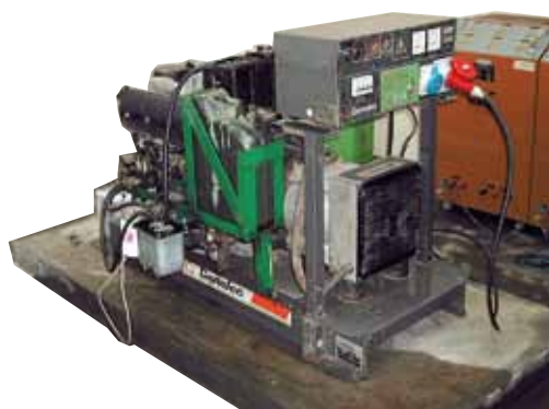
Testing a diesel motor fueled with vegetable oils in the 2IE biofuel laboratory in Burkina Faso
