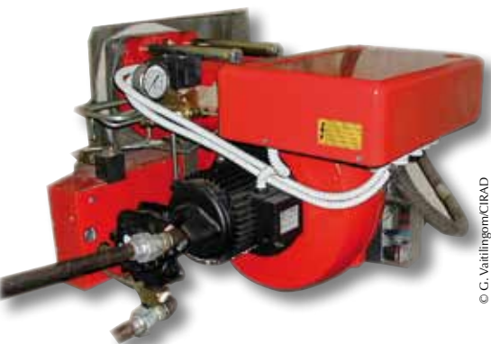
The CIRAD-Riello boiler using palm oil to dry rubber in Cameroon
