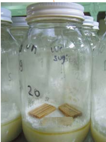
Measuring the resistance of treated wood to wood-rotting fungi © F. Lyon
