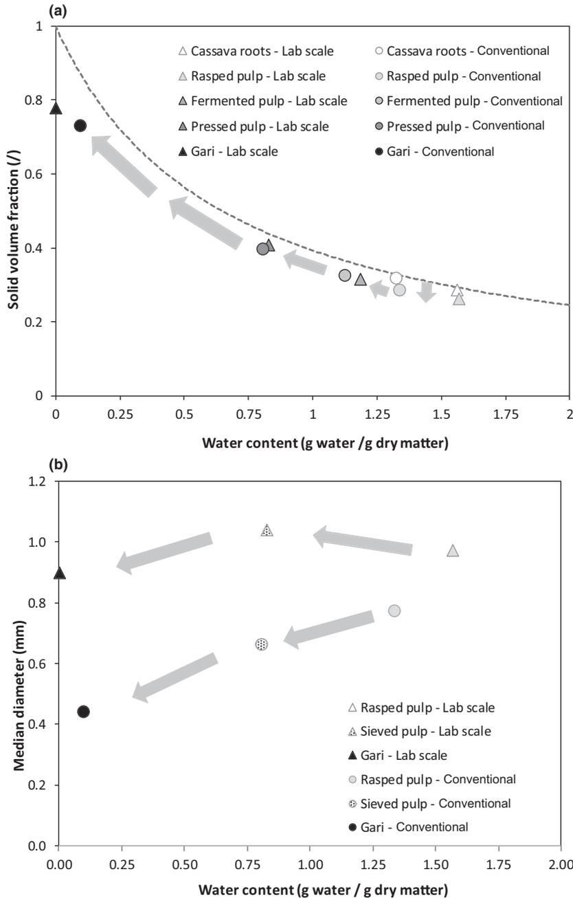
**Figure 3** Hydro-textural diagram showing the evolution of solid volume fraction (a) and median diameter (b) vs. water content during gari processing by conventional process (○) and laboratory-scale process (△).
