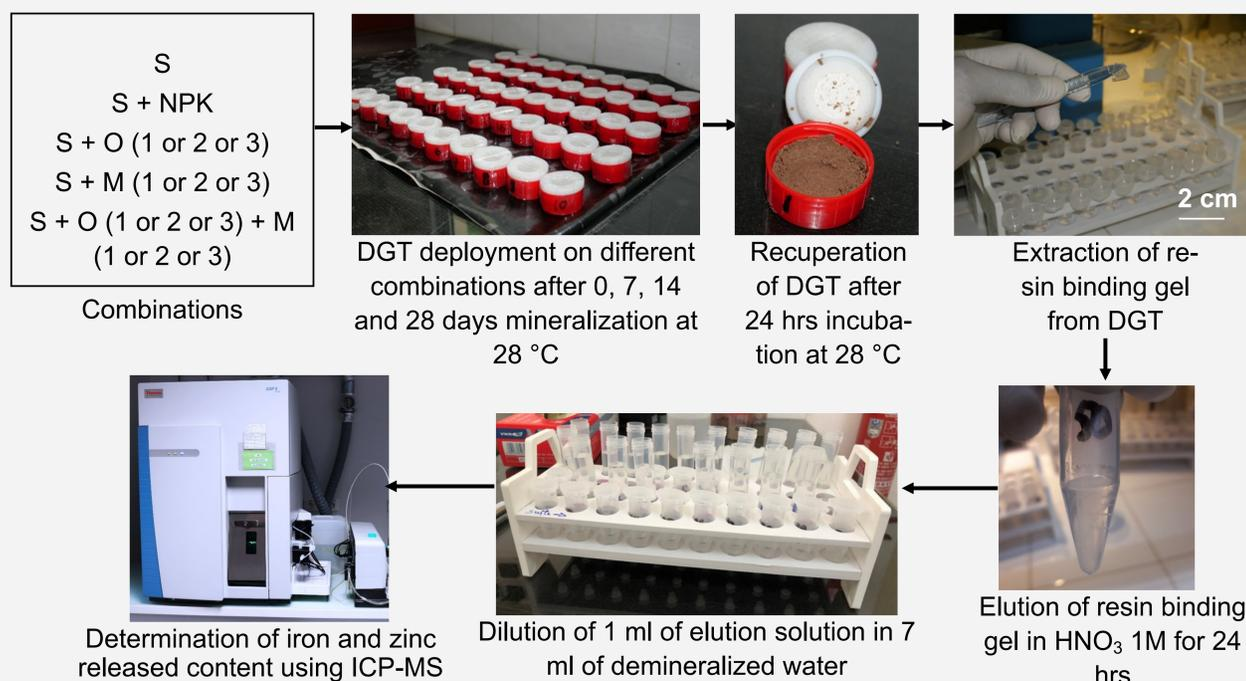
S = soil; O1 = cow dung; O2 = poultry droppings; O3 = sewage sludge; M1 = Saint Louis (peanut + millet); M2 = south groundnut basin (peanut); M3 = south groundnut basin (rice); ICP-MS = Inductively coupled plasma mass spectrometry
