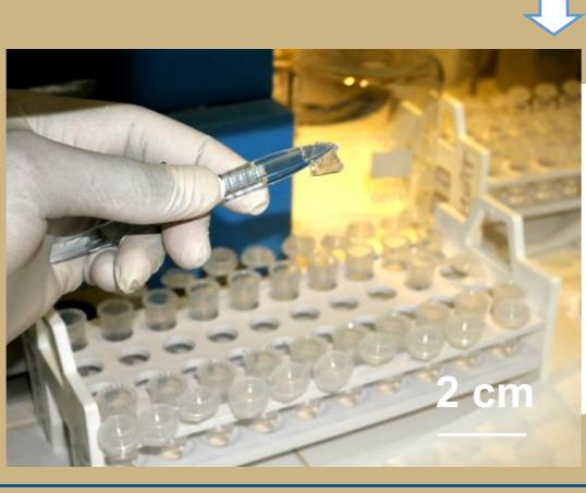
Extraction of resin binding gel from DGT
