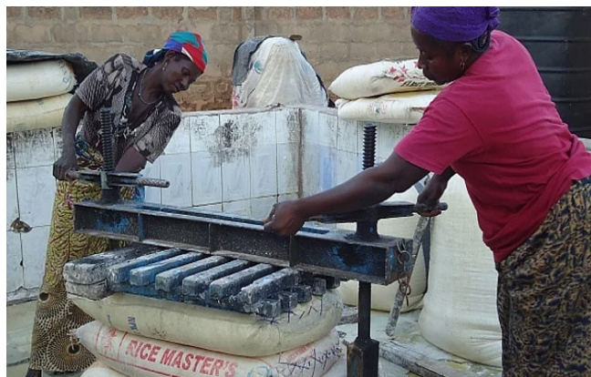
Figure 6: Dewatering of cassava mash
